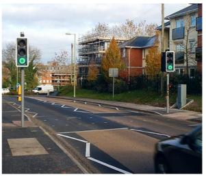
In addition, they are used at sites with high pedestrian flows to reduce delays to traffic by grouping pedestrians.
